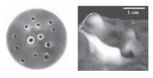
5-mm depth of the fluid and extended to the bottom of the container, which was 9.4 cm across. The researchers attribute the holes' stability to shear thickening—an increase of viscosity with shear rate. At higher accelerations, as shown in the side view (right) of a single hole, the rim grew fingerlike protrusions that rose 2 cm above the surface and undulated erratically. (F. S. Merkt *et al.*, *Phys. Rev. Lett.* **92**, 184501, 2004.)
