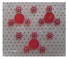
net activity, the overlying rotors can be put into new arrangements for carrying out a new job (*See figure*). The rotors are at the millimeter scale but can be made much smaller. Unlike conventional machines the rotor arrays have no fixed axles and are virtually friction free. (Grzybowski *et al., Appl. Phys. Lett.* **84**, 1798, 2004)
