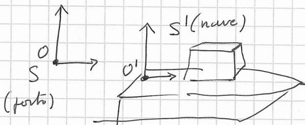
$$\begin{aligned} \vec{r}' & (\vec{r}') \\ \vec{v}' & (\vec{V}') \\ \vec{\alpha}' & (\vec{\alpha}') \\ \vec{r} & = \vec{r}' + \vec{R} \quad \vec{R} = \vec{OO}' \end{aligned}$$
